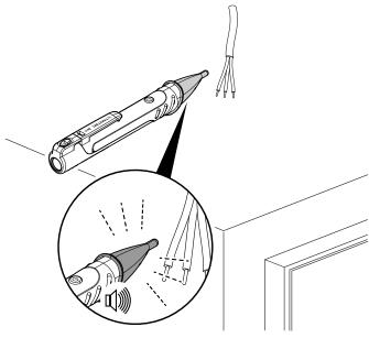
⇒ If there is an AC voltage within the selected sensitivity range present at the source, the measuring tip (7) will flash and a repetitive beep will be emitted.
